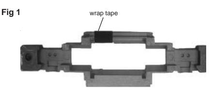
wrap tape the whole notch with tape to prevent the motor's spring contact from touching the chassis. Otherwise the decoder will be destroyed if the motor contact touches unwrapped part of chassis
